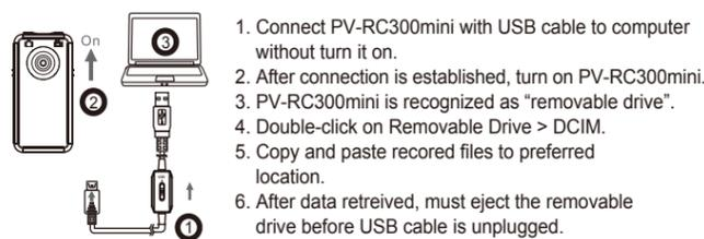
1. Connect PV-RC300mini with USB cable to computer without turn it on.
