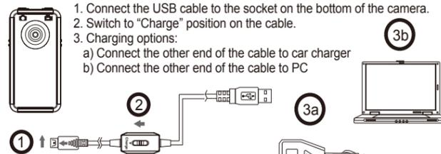
1. Connect the USB cable to the socket on the bottom of the camera.
