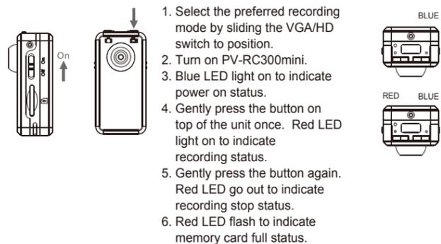
1. Select the preferred recording mode by sliding the VGA/HD switch to position.
