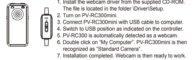
1. Install the webcam driver from the supplied CD-ROM. The file is located in the folder \Driver\Setup.
