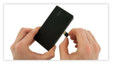
To install the micro SD card, place the camera on a flat surface with the BrickHouse Security logo facing down. The card should be inserted with the gold contacts facing up, away from the logo.
